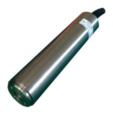
**FA7-BA** Cyanobacteria (Blue-green Algae) sensor uses fluorescence approach to measure cyanobacteria concentrations in water. When cyanobacteria are excited by a high-energy LED light source of 590nm, it produces a specific wavelength fluorescence which based on its spectrum absorption characteristics, can be used to detect cyanobacteria concentrations in water.
